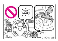
Vehicles with a Multidrive: Check that the shift lever is securely set in P. The engine may not start if the shift lever is displaced out of P. The smart entry & start system indicator light (green) will flash quickly.
