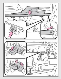
Pull the rubber strip on the edge to unhook it from the cover, and then push the tabs in and lift the cover off. Remove the battery terminal cover and then the fuse box cover.
